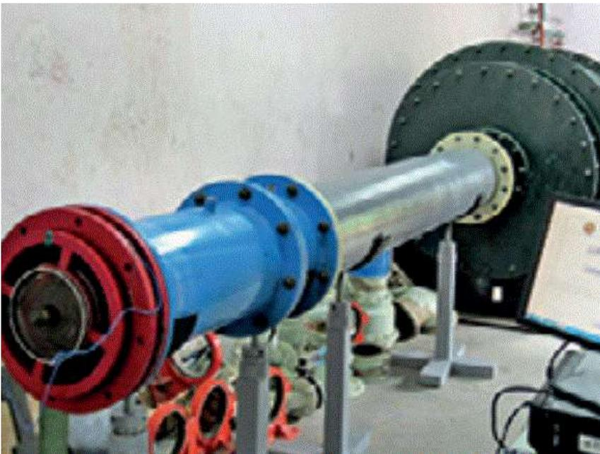
CHENNAI: A team of 25 faculty members and students from the ocean engineering department in Indian Institute of Technology Madras have begun testing a prototype of a turbine they have developed which converts wave energy into electricity. The 'impulse' turbine works with a unidirectional rotor powered by a generator. The system will be tested in oceans by the end of the year.
