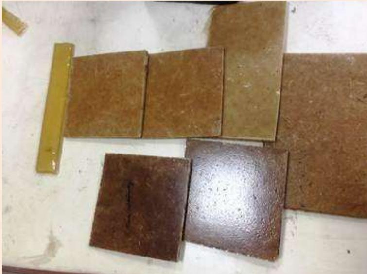
Tiles developed by IIT Researchers using waste including plastic.
